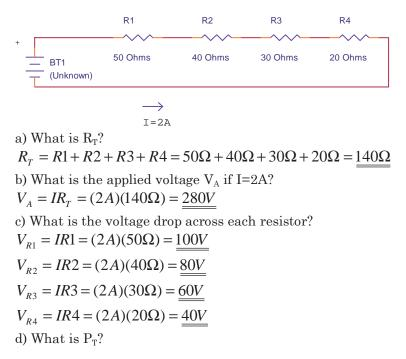
$P_T = V_T I = V_A I = (280V)(2A) = \underline{560W}$  (Can also be found by  $I^2 R_T$ ) e) What power is dissipated by R2? By R4?
