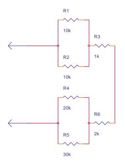
$R_{T} = (R1 \parallel R2) + R3 + R6 + (R4 \parallel R5) = 10k \parallel 10k + 1k + 2k + 20k \parallel 30k = \underline{20k\Omega}$
