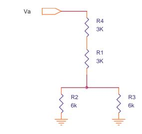
$R_T = R4 + R1 + (R2 \parallel R3) = 3k + 3k + (6k \parallel 6k) = \underline{9k\Omega}$
