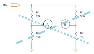
(Again, the four resistors should be labeled R1-R4). For any bridge, the product of the "cross arms" is set equal:
