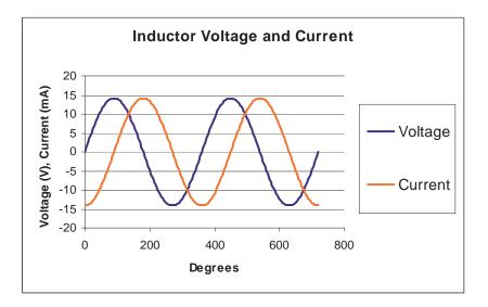
The voltage leads the current by 90 degrees in an inductor.
