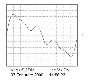
Ch 1: Laser Drive Voltage at Q3 Collector
