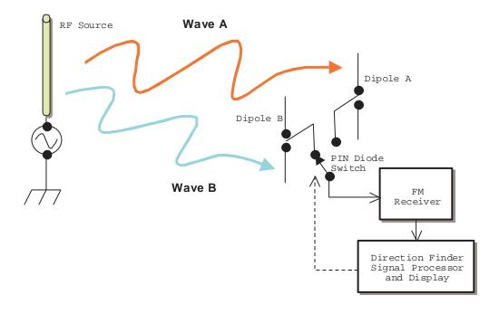
Figure 1: Doppler method with two antennas
