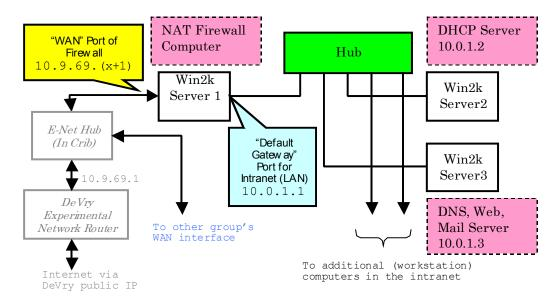
In the picture above, E-Net Hub is in the electronics laboratory stockroom. The jumpers at the end of your lab bench connect to this hub. *You have to request that the crib connect the bench to the experimental network*. Once this has been done, the bench connection that would normally go to the DeVry University intranet now connects to the experimental network.
