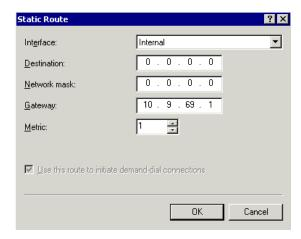
In the figure above, the destination network is 0.0.0.0 (any), and the gateway is 10.9.69.1 (E-Net gateway). When the firewall computer receives a packet bound for an unknown network, it will automatically forward this packet to *its* default gateway at 10.9.69.1.
