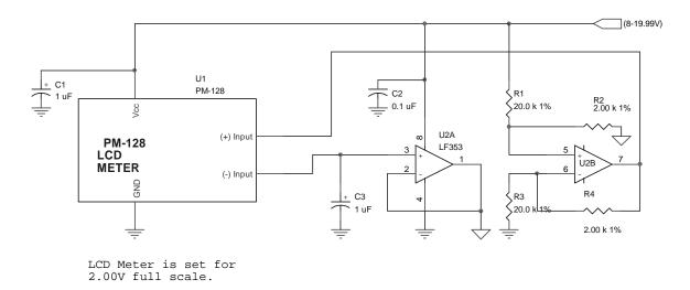
Figure 2: Power Supply Monitor Circuit
