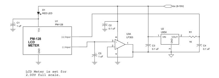
Figure 1: LCD Electronic Thermometer Circuit
