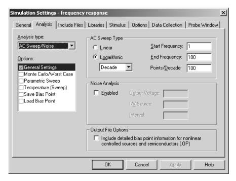
This profile will sweep any AC sources in the circuit from 1 Hz to 100 Hz (two decades), with 100 points for each decade.
