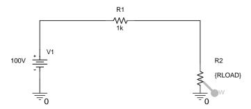
2. Place a new part on the drawing called "PARAM" (from the SPECIAL library.) Place it on the schematic, then double-click its body to open its property sheet.
