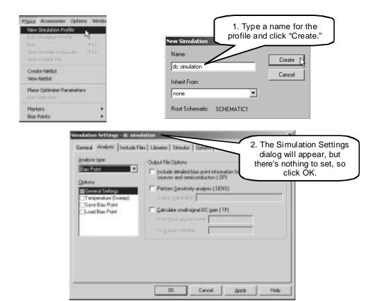
You can have multiple profiles for a given project. This allows you to analyze a circuit in different ways without having to change settings back and forth.
