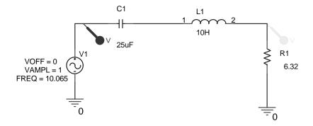
This modification raises the resonant frequency of the circuit to 10.065 Hz, and the Q becomes 100.
