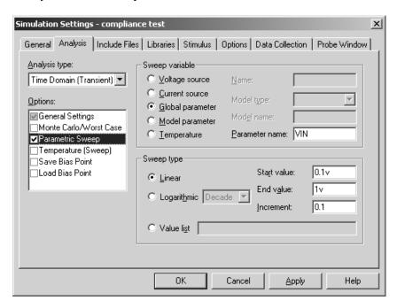
To set this up, *first* click on the checkbox by "Parametric Sweep" in the Options window. Then fill in the fields on the right as shown.
