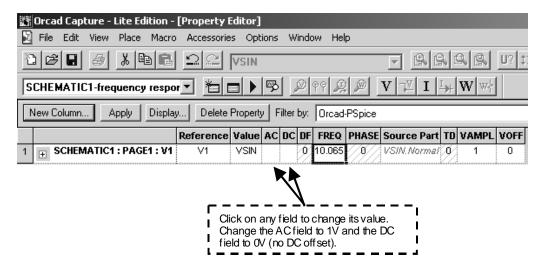
This screen is available for all components in a design. Not all of the parameters display on your drawing because the display isn't turned on for them. To fix that, highlight one of the items, then click the "Display..." button. Choose "Name and Value" from the dialog to make the parameter show on the drawing.
