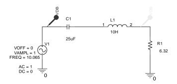
9. With these special probes in the circuit, run the analysis again. Notice that we played a dirty little trick. By setting the input voltage to 1 V (0 dBV), we get output voltage magnitude readings that correspond to the voltage gain.
