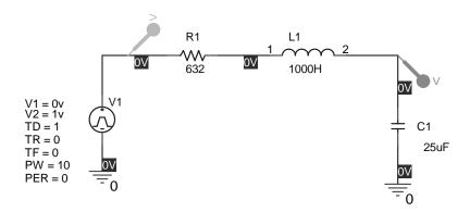
Place the two voltage probes by clicking the probe button on the toolbar. Note the *color* of each probe; it will match the color of the trace in the PROBE readout during simulation.
