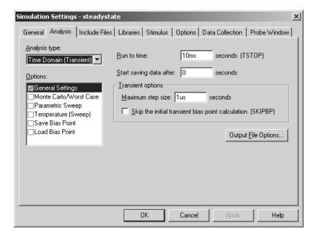
Note that the VSIN source in the circuit is set to 1 KHz, and that the analysis steps are  $1 \mu S$  -- so there will be 1000 calculations for each sine wave cycle. With the TSTOP setting of 10 mS, we should see 10 cycles of the waveform on the display.
