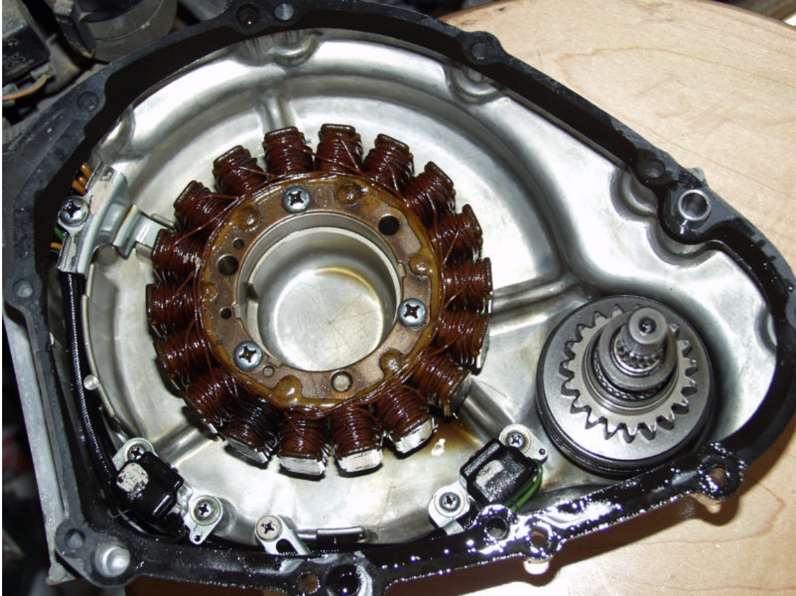
Figure 1 : Stator Mounted in Engine Cover.
