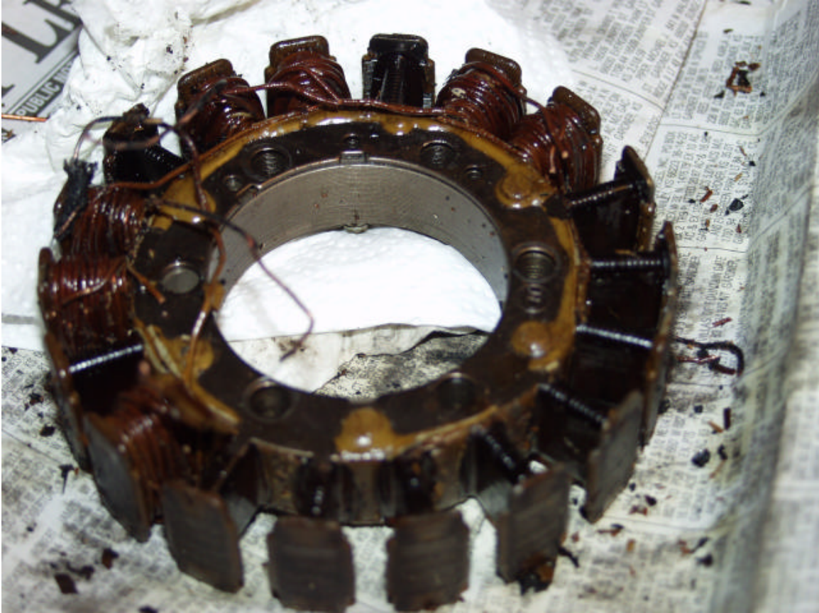
Figure 2: The Removed Stator on the Bench, Partially Disassembled
