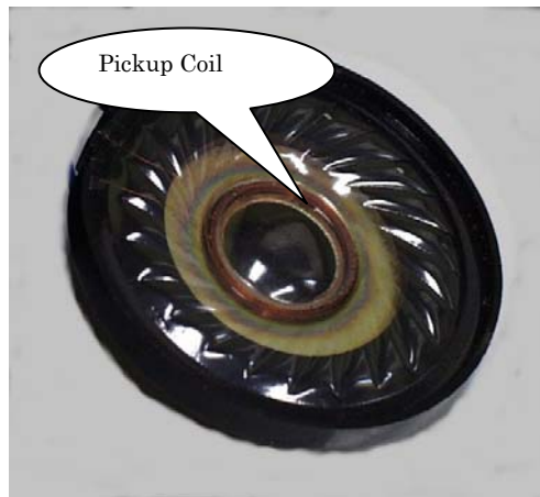
Figure 1-2: A Typical Dynamic Microphone Element
